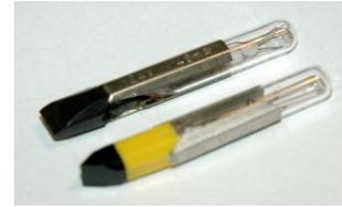
Standard GPO bulb 24v in the lower current rating 40 ma or 60ma. To save cooking the buttons!
