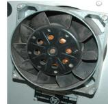
Vintage **Papst 5 inch fan** 115v or 230v. These all metal fans were common in the 60's but now are prone to bearing failure & noise. Again looking for correct type for originality. Used a lot and need several
