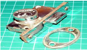
These are the Yale locks that are fitted to the side lockers. Some of the original ones are there but all are in poor corroded condition. Possibly Yale type 229 or M69
